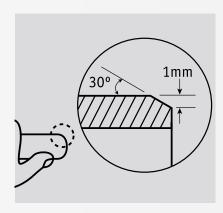
Check the tube ends are free from damage and clean, wiping away any swarf to avoid damaging the 'O' ring on tube insertion. Tube end must also be free from stickers, tape and adhesive residues.
