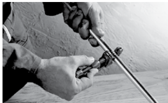
FIGURE 1: CUTTING THE TUBE
