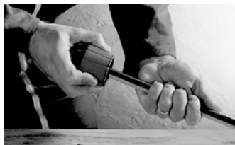
FIGURE 2: DEBURRING THE TUBE
