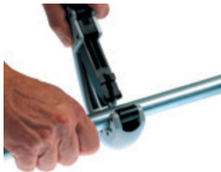
FIGURE 4: CUTTING THE TUBE
