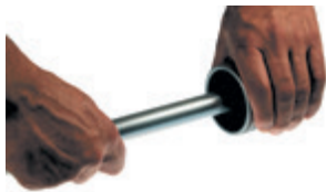
FIGURE 5: DEBURRING THE TUBE
